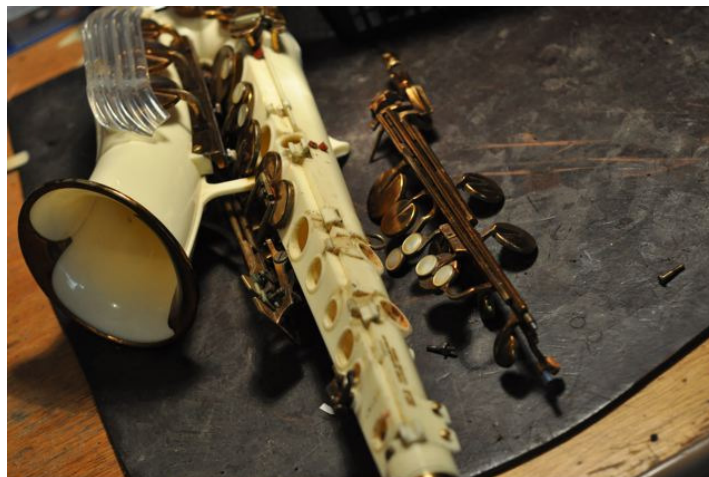
Saxophone with the upper stack of keys and pads removed.
